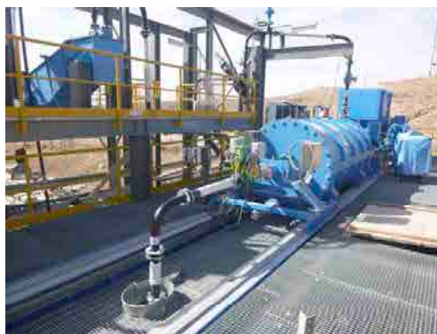
Figure 2 – IsaMill grinding circuit.
