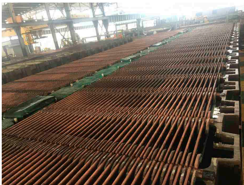
Figure 2. ISAPROCESS™ permanent stainless steel cathode plates in service.
