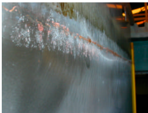
Figure 4: Solution line corrosion
