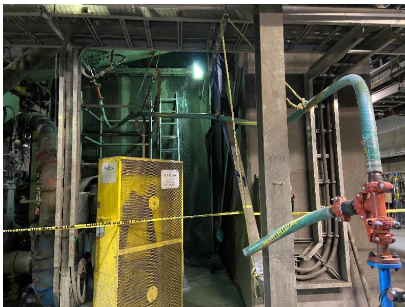
FIGURE 8: FEED ARRANGEMENT TO M100 ISAMILL™
