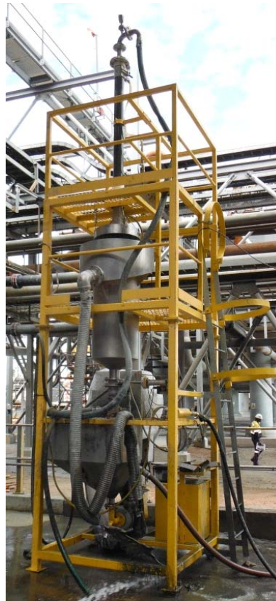
Figure 6 – Jameson Cell L500 pilot plant test rig at Lumwana site
