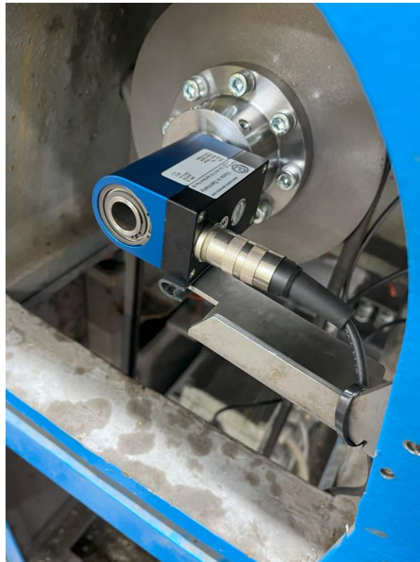
Figure 4: Torque Sensor installed on an M4 IsaMill™ Shaft
