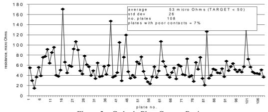
Figure 2 – Cathode Plate Contact Resistance
