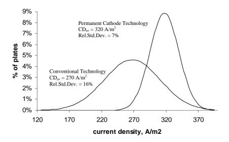
Figure 1 – Current Distribution Comparison - Conventional and Permanent Cathode
