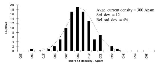
Figure 3 – Measured current distribution data, ISA PROCESS<sup>TM</sup> tankhouse (7)
