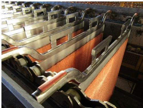
Figure 5: ISAKIDD Steerhorn Cathode with top-mounted shorting frame contacts
