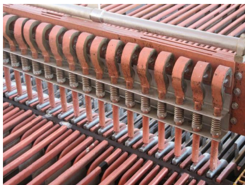
Figure 6 Spring-contact shorting frame in operation with IK cathode bars employing
