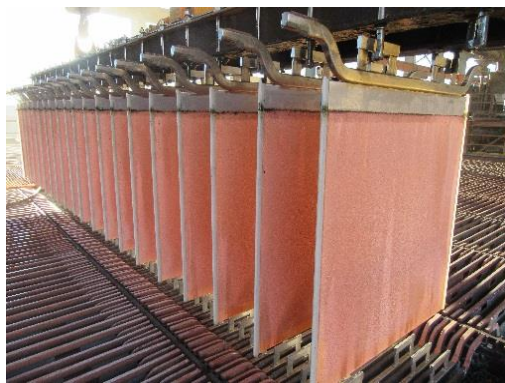
Figure 2 ISAKIDD Steerhorn Cathodes in service
