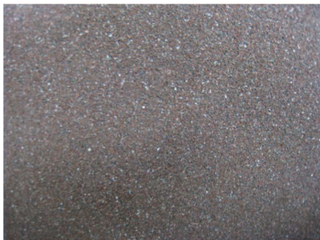
FIG 11 - Regrind fresh feed oversize screened at 300 microns.
