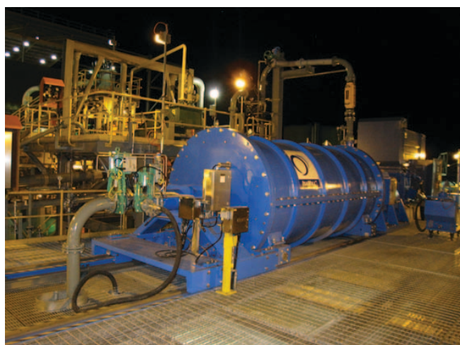
FIG 5 - The Ernest Henry Mine 3 MW M10 000 IsaMill.
