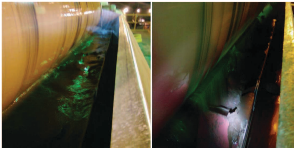
FIG 10 - Regrind magnetic separator sanded (left) and with tailings valves open (right).
