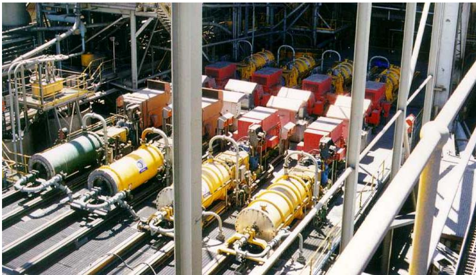
Figure 1: IsaMills in the Regrind Circuits at the Mount Isa Mines Lead/Zinc Concentrator
