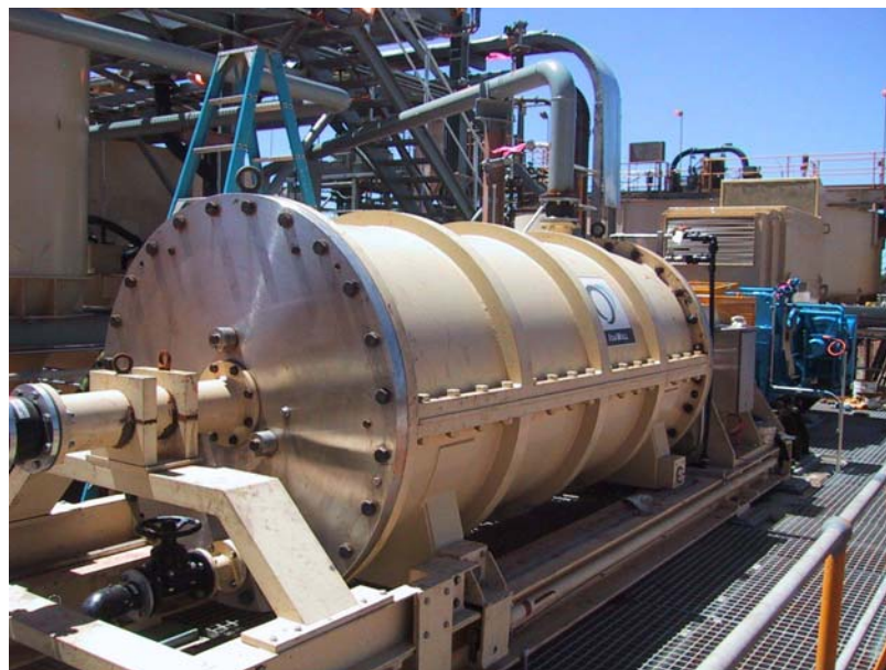
Figure 15: IsaMill with a Split Shell Design
