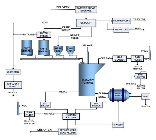
Figure 1- Britannia Refined Metals Secondary Operations Flow sheet
