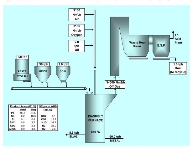
Figure 6 - Process Flows for a 300,000 tonnes per year Secondary Lead ISASMELT<sup>TM</sup> Plant
