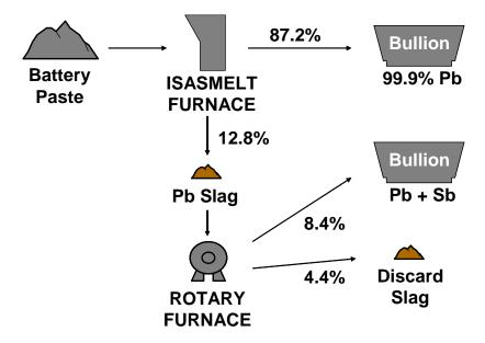
Figure 2-Lead Distribution in the BRM Process
