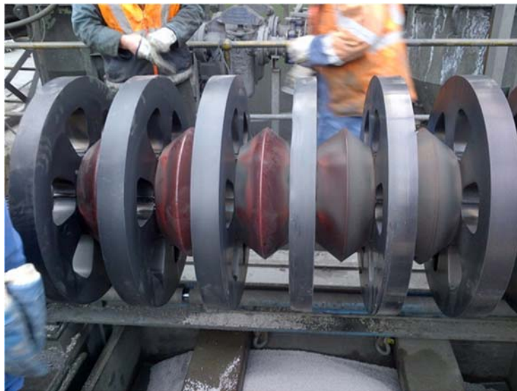
Figure 7 - M1000 IsaMill™ configured with conical spacers
