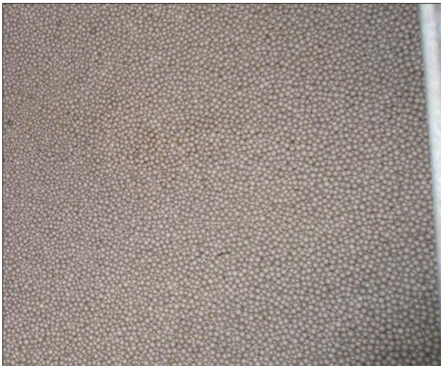
Figure 8. Cenotec 6.5mm ceramic media charge at EHM after 1 month (Larson 2011)
