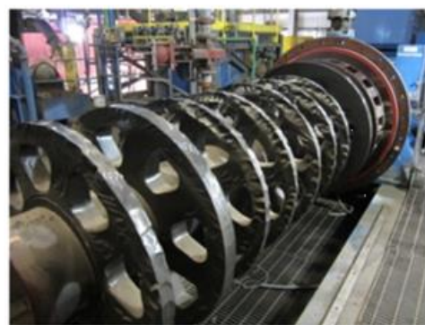
Figure 5 – IsaMill small diameter disc installation from discharge (left picture) and feed (right picture) ends
