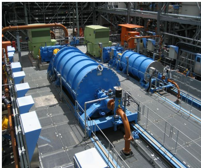
Fig. 10. – Amandelbult UG 2 IsaMills™ showing MIG and UFG concentrate regrind mills.
