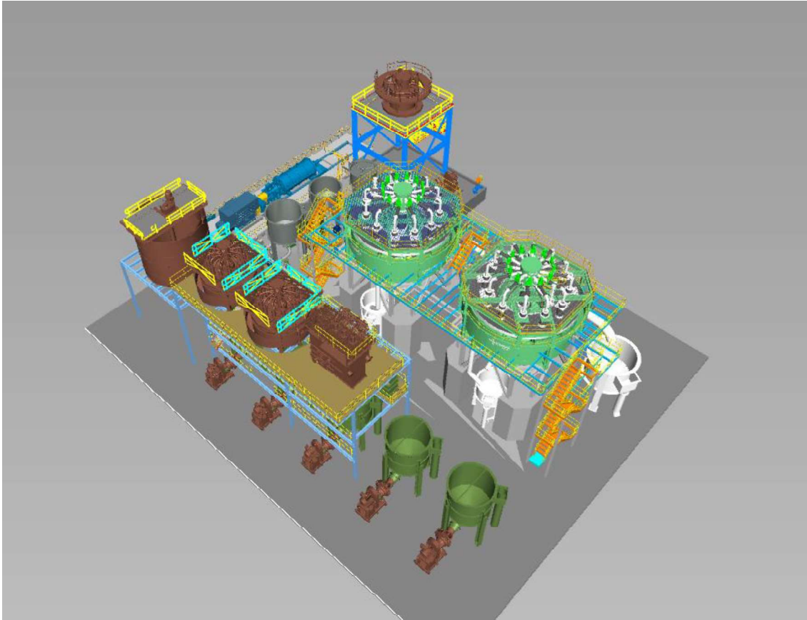
Figure 5: Plant Layout - Jameson Concentrator
