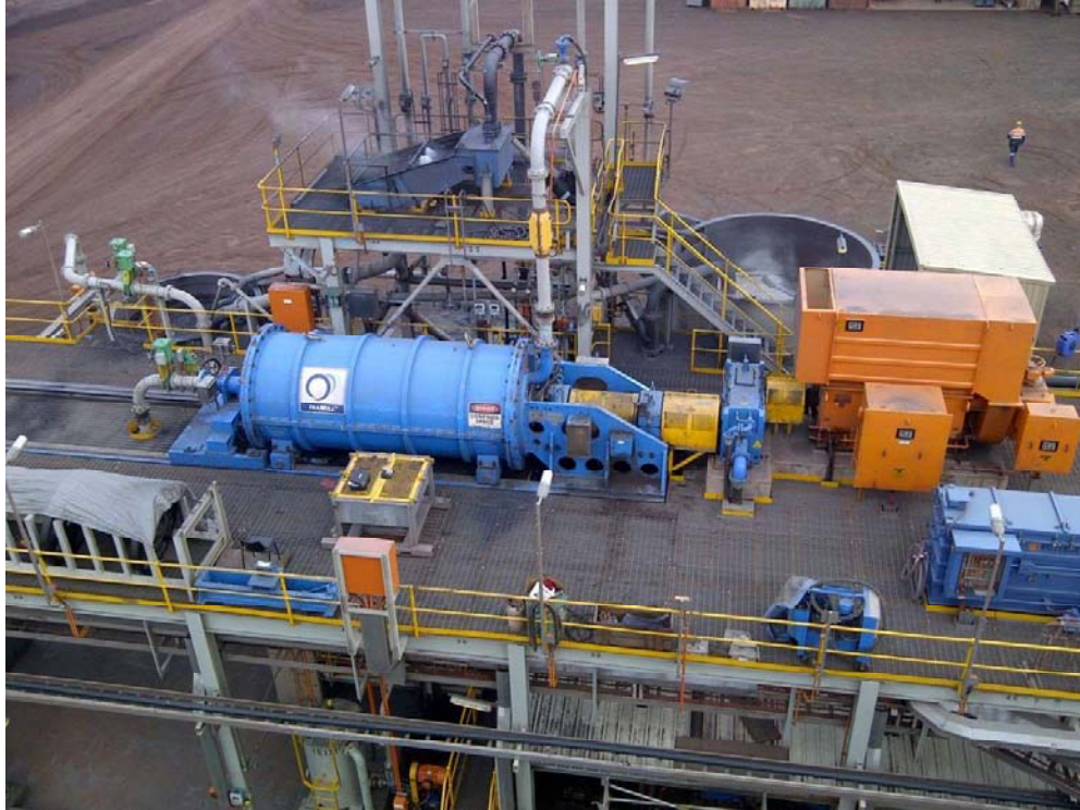
Figure 6 – Arrium M10000 IsaMill installation.
