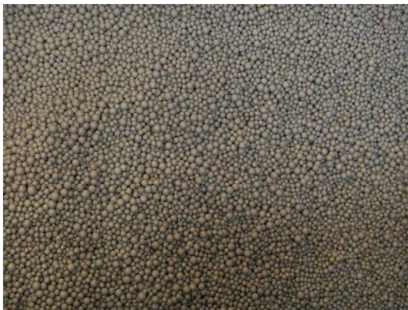
Figure 10 – Arrium IsaMill graded media charge.
