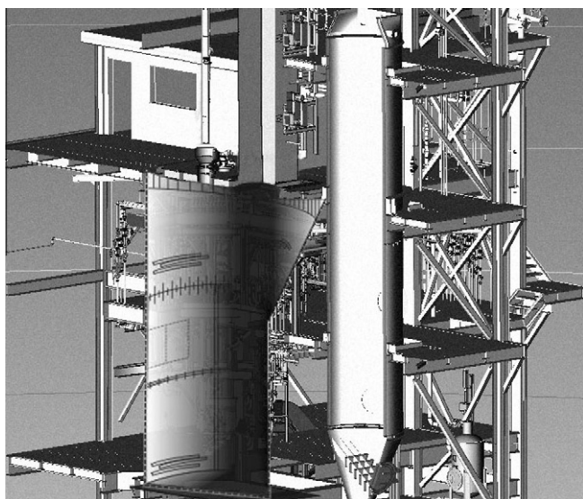
Fig. 4. Cutaway of a design for the ISACONVERT™ furnace.
