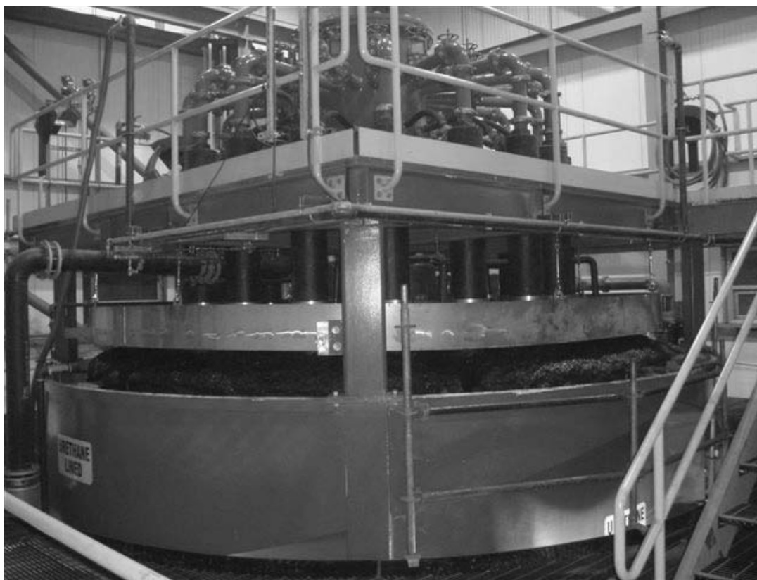
Figure 6: The preflotation Jameson Cell during commissioning at Red Dog Mine.
