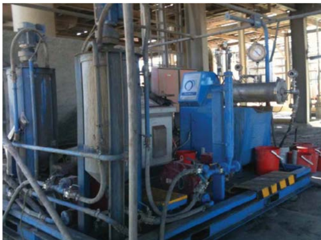
FIG 10 - Pilot ISAMill M20 used for both copper and pyrite regrind circuit development and scale-up.
