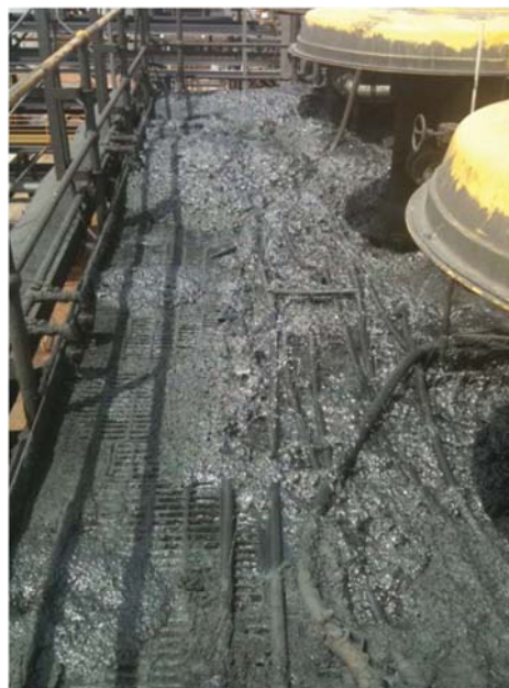
FIG 6 - Photograph of overloaded Train 2 reCleaners prior to Jameson cell installation.
