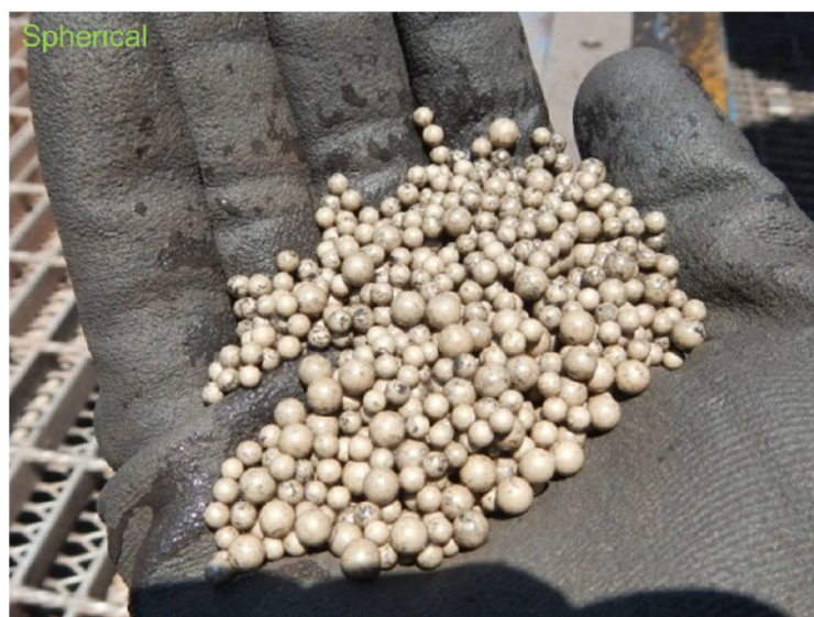
Figure 7 – Uniform Grinding Media Wear (Glencore Technology, 2018a)
