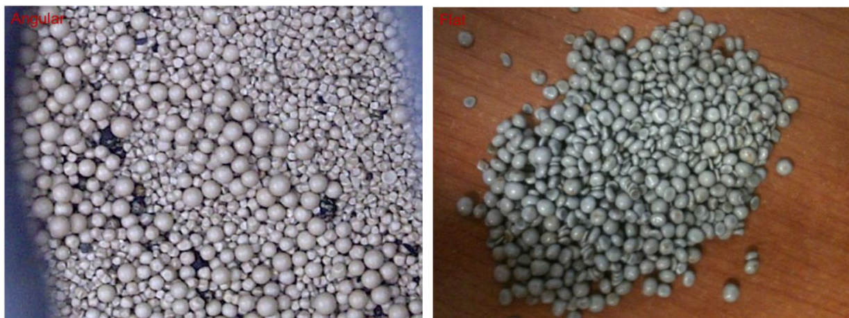
Figure 8 – Non-Uniform Grinding Media Wear: Angular (left), Flat (Right) (Glencore Technology, 2018a)
