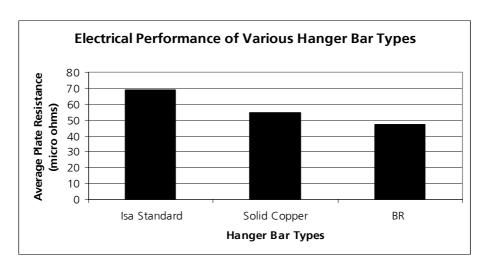
Figure 2 – Internal resistance of various hanger bar types
