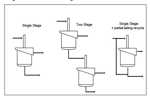
Figure 1 - Jameson Cell configurations for fine coal flotation
