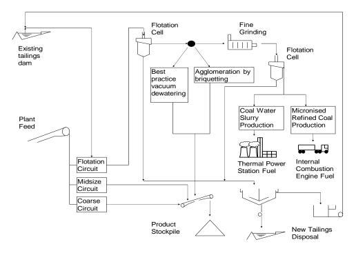
Fig. 5 Alternative fines treatment for thermal coals
