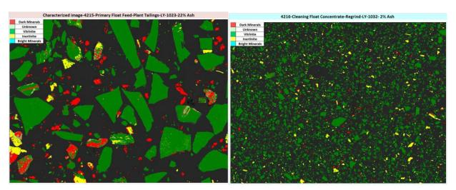
Fig 2 Characterised images for raw coal tailings feed and final concentrate (courtesy QCAT-CSIRO)
