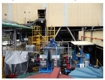
Fig. 3 The 3 t/day coal tailings treatment pilot-plant (Courtesy Glencore)
