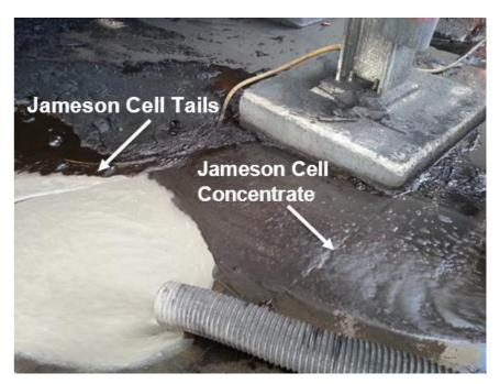
Fig. 4 Concentrate and tailings streams from pilot plant test-work (courtesy Glencore)
