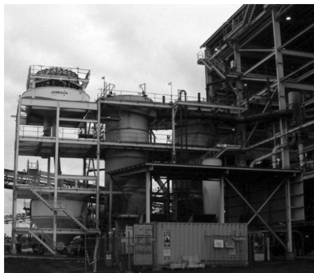
Figure 8: Recently installed Jameson Cell (left) next to two column cells at AAMC's German Creek operation
