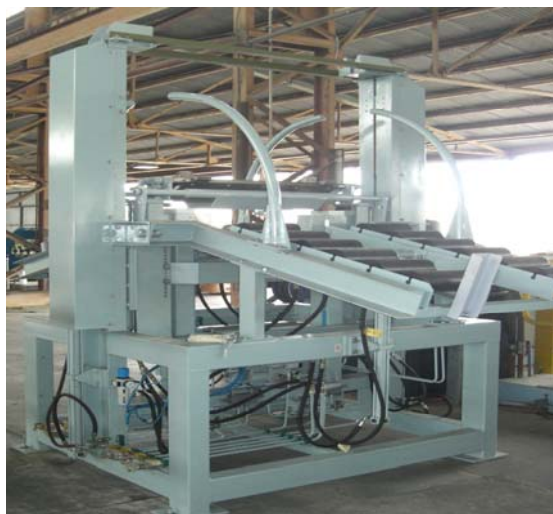
Figure 6 – ISA 2000 Flexor Stripper
