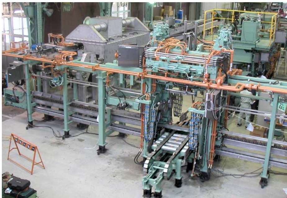
Figure 3 – ISA 2000 Waxless machine stripping station
