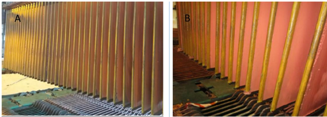
Figure 12. Overlap tests with 20 mm in Cell 1. A: cathodes before the test; B cathodes during the test
