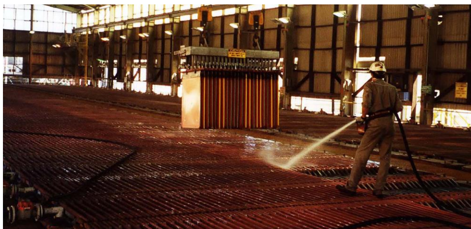
Figure 3 – Block stripping the “A” cathodes in three cells.
