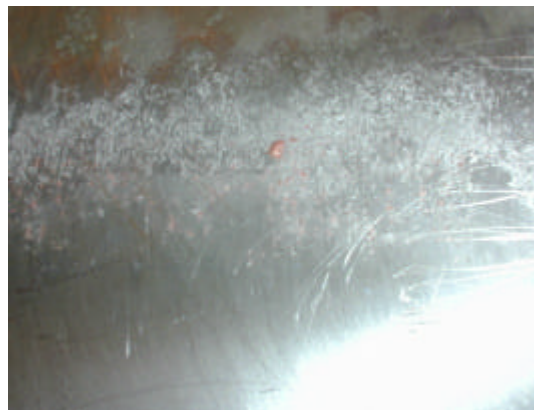
Figure 3: Surface corrosion of the cathode mother plate
